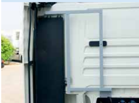
Handy: the condenser fastening frame uses the vehicle's existing fastening points.
